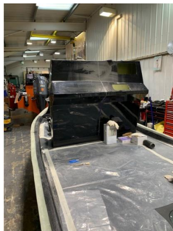
FPV Vigilant with console in position and engines fitted
