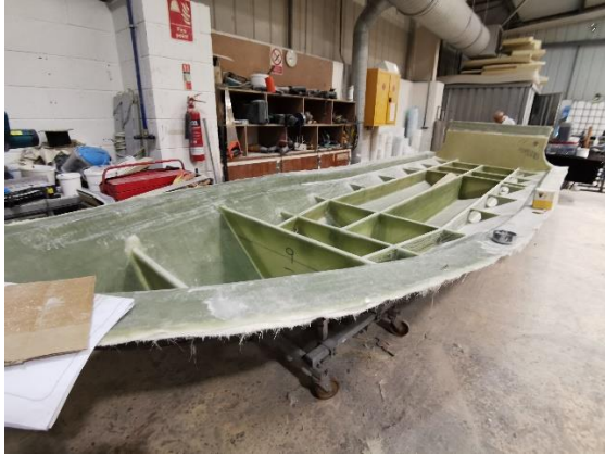
The hull of FPV Vigilant prior to installation of the fuel tanks (right)
