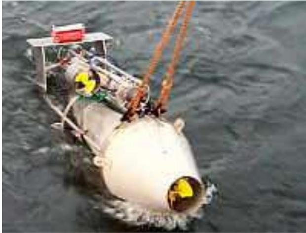
Fig.6 towed plankton recorder used by Cefas for fish egg surveys.
