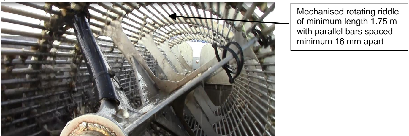
Figure 6. Cockle suction dredge (a) and sorting riddle (b)
