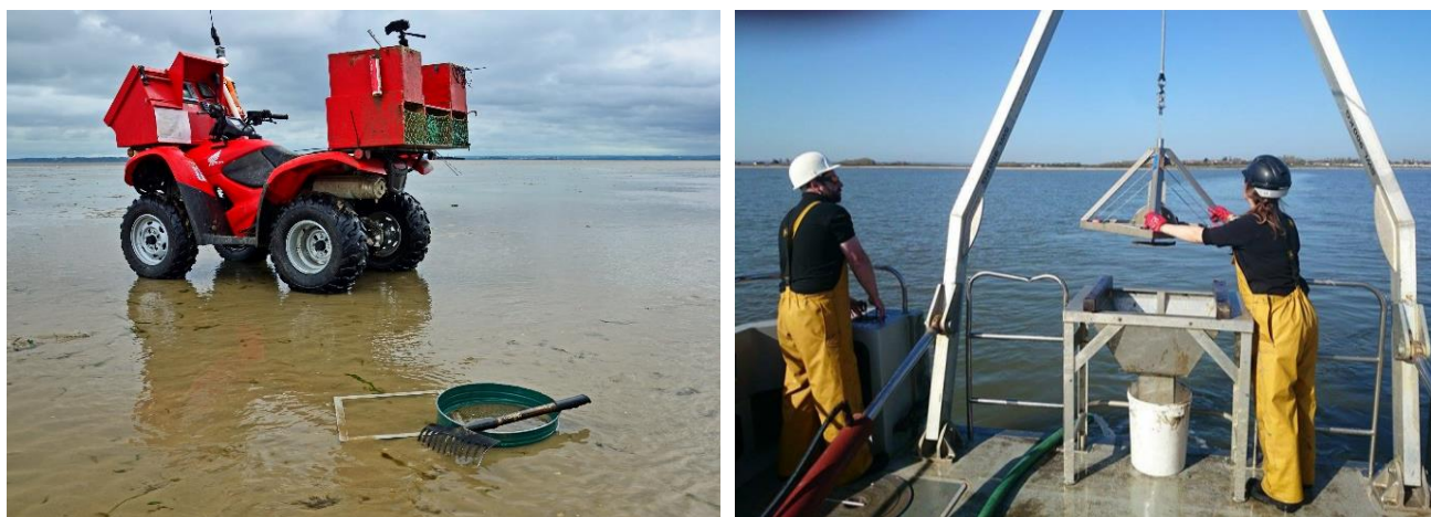
Figure 2: Sample collection methods; (a) ATV, quadrat, rake and sieve; and (b) Day grab deployed from vessel.
