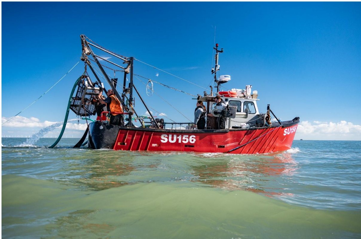
Figure 1. Manila clam trial fishery participating vessel, Audacity, showing the water injection batch dredge lowered from the back of the vessel in the Thames Estuary, 2024. Photo credit: Colm O'Laoi.
