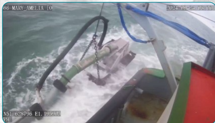
Above: REM CCTV footage of a cockle dredge being brought back to the surface at the end of a fishing operation. A sensor attached to the dredge head sends a message to KEIFCA to notify that fishing activity has stopped.
