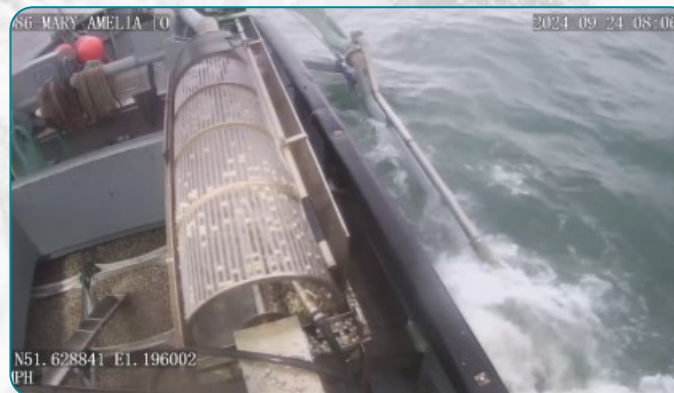
Above: REM CCTV footage showing cockles passing along the riddle and into the hold. Future management approaches may be able to use this to incorporate fine-scale spatial management measures that have not been possible until now.
