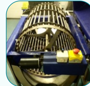
Above: KEIFCA's compact battery-powered rotary riddle was lent to fishermen to try out.
