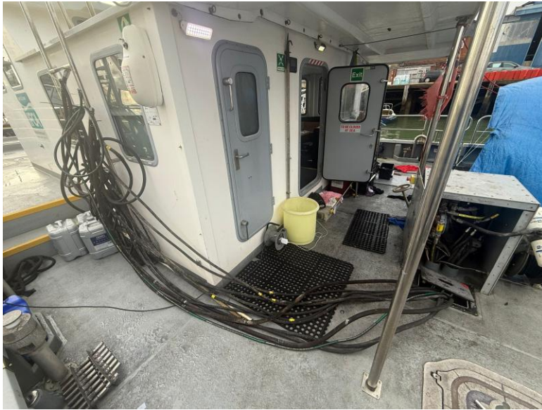
Old hydraulic hoses being removed at Diverse Marine
