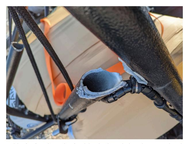
A debriefing from this incident found that the skipper had acted appropriately and that this was an unforeseen incident due to a welding issue on the A frame . The A frame structure has been subsequently repaired by the manufacturers, Ribcraft, with some modifications. Although the warranty period had ended, Ribcraft agreed that this was not something that would normally be expected to occur on a vessel less than 2 years old and carried out the repair free of charge.
